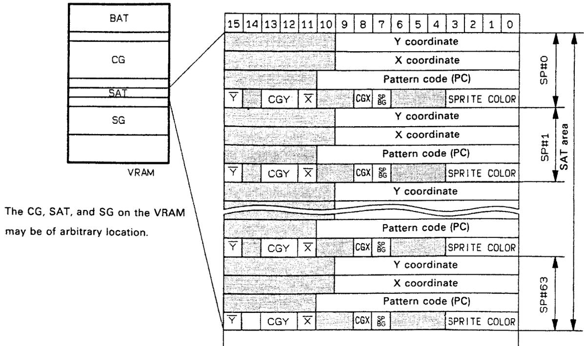
In the SAT area, four words are used to define one sprite (256 words to define a total of 64 sprites). The priority of sprites follows that of addresses.
