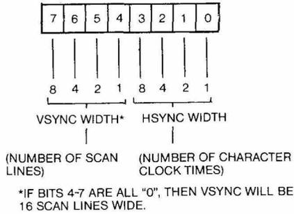
Control of these parameters allows the 6545-1 to be interfaced to a variety of CRT monitors, since the HSYNC and VSYNC timing signals may be accommodated without the use of external one-shot timing.
