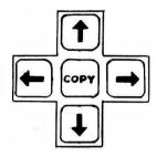
Hold the pen very steady and press the respective directions to move the cross under the tip of the pen. Press <ENTER> to record this new setting or <ESC> to leave the setting unchanged. You can recalibrate at any time during using the program,
