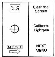
The first ikon will clear the screen's contents and should be carefully used! The second allows you to enter the lightpen calibration routine. Point the lightpen at the calibrate ikon and press (ENTER) to confirm your choice.
